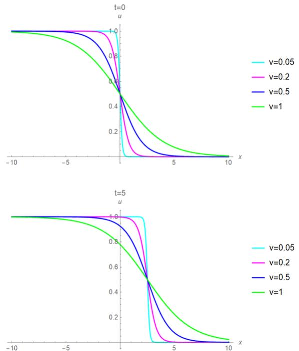
Figure 2. Different right-moving, kink-shaped solutions of the viscous Burgers equation, for  $\nu \in \{0.05, 0.2, 0.5, 1\}$  and  $\lambda = 0.5$ , on the interval  $x \in [-10, 10]$  and with  $t \in \{0, 5\}$ . Small viscosity effects lead to a steeper waveform, whereas larger viscosity effects lead to smoother and wider waveforms.
