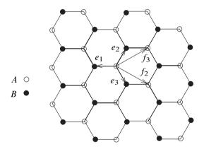
Figure 7. The honeycomb lattice  $\Lambda_{hon}$ , the generators  $f_i$  for  $L(\Lambda_{hon})$  and the generators  $e_i$  of  $T(\Lambda_{hon})$ .
