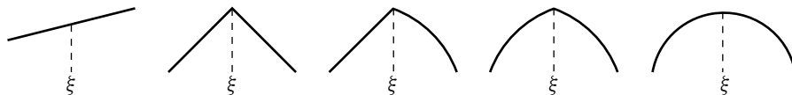
Fig. 2.1. In the first three graphs, g is not strictly concave at \xi while in the last two it is.
