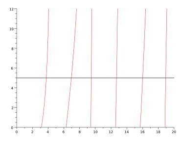
Figure 2. Top: the first eigenfunction of A, i.e. the fundamental mode of resonance of the flute with an open hole. Bottom: the graphic of the function  $f_a$  and the intersections with the line  $y = \alpha \delta$  giving the frequencies of the flute. The references values are a = 0.7 and  $\alpha \delta = 5$ .
