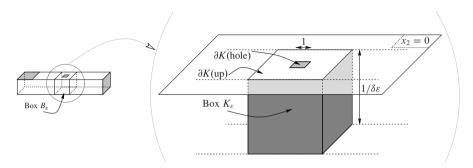
Figure 3. The cube  $K_{\varepsilon}$ , part of the half-space  $K = \{x \in \mathbb{R}^3, x_2 < 0\}$ , and the corresponding boundaries. When  $\varepsilon$  goes to 0, the cube  $K_{\varepsilon}$  converges to K, whereas the hole  $\partial K$  (hole) remains unchanged.
