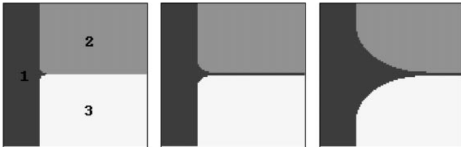
FIG. 9. Simulation of an unstable trijunction at time steps t = 0.0005, 0.0200, 0.0300 .
