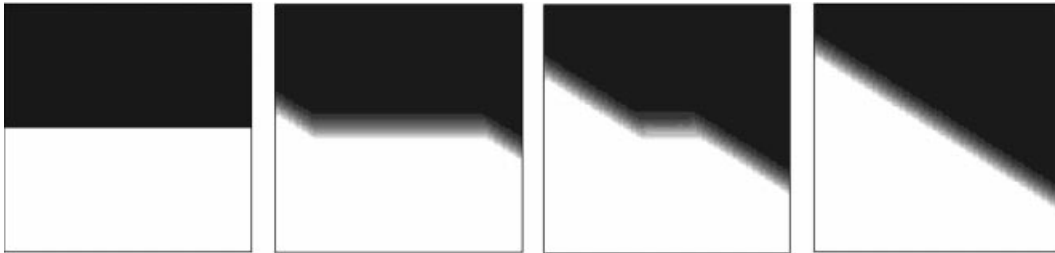
FIG. 12. Crystalline interface shown at time steps t = 0.00, 0.05, 0.30, 0.55 .
