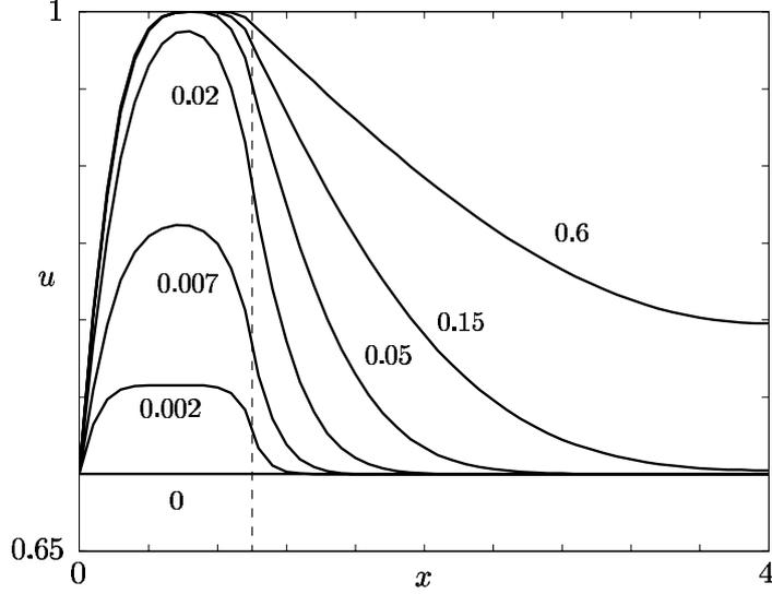
FIG. 3. Evolution of dimensionless salinity  $u$  for root distribution  $k(z)$  given by (2.14), and for parameter values  $p = 0.5$ ,  $k_0 = 15$ ,  $d = 4$ , and  $u_0 = 0.7$ . Numbers in the figure are values of  $t$ .
