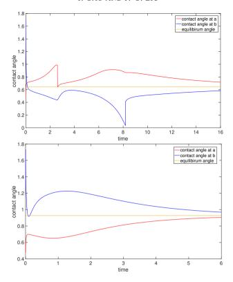
FIG. 4. The contact angle dynamics for the associated droplets dynamics in Fig. 3. (Left) Evolution of contact angles for  $t \in [0, 16]$  for the rolling down case with  $\sigma = -0.8$ ; two cusps when the advancing (resp. receding) contact line a(t) (resp. b(t)) passing through the corner between the mouth and the body of the teapot. (Right) Evolution of contact angles for  $t \in [0, 6]$  for the rising up case with  $\sigma = -0.6$ .
