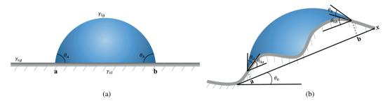
FIG. 1. (a) Illustration of contact angles  $\theta_a$ ,  $\theta_b$ ; (b) Illustration of contact angles  $\theta_a$ ,  $\theta_b$  and the local slopes of the rough surface  $\theta_{0a}$ ,  $\theta_{0b}$ .
