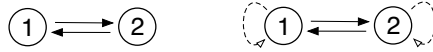
Figure 6. Two 2-node networks with different network topologies that define the same space of admissible maps. Left: \mathcal{G}_1 . Right: \mathcal{G}_2 .
