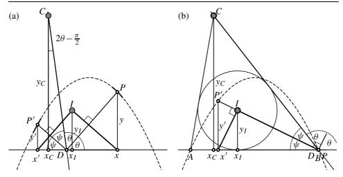
machine then produce the two angle bisectors at D (which are mutually orthogonal) and project the point I orthogonally to these bisectors onto the x-axis, producing the abscissas x and x', respectively. Then the corresponding points P and P' on the bisectors move on one and the same parabola with vertical axis.
