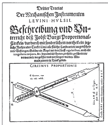
Fig. 3 Bürgi's "Proportional Circel", a precision compass device invented and built by Jost Bürgi, first mentioned by Levin Hulsius in 1603 (published in 1607). It serves to reduce the scale of an object by a constant factor (from [19], p. 130).
