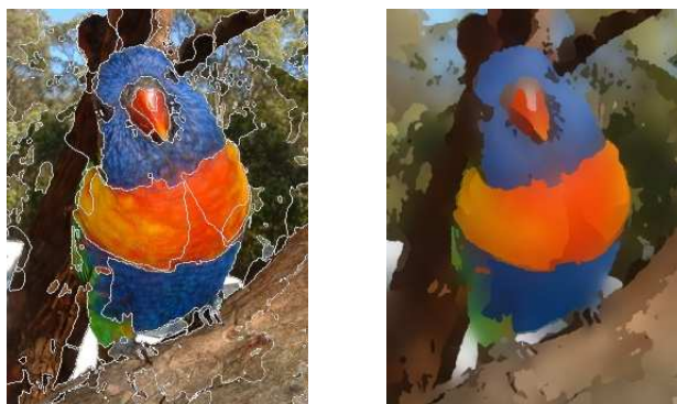
FIGURE 1. segmentation of a RGB image, original with boundaries (left), piecewise smooth approximation (right)
