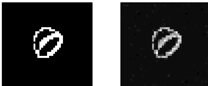
FIGURE 1. True activity function (left) and optimal reconstruction from degraded data with 10% Gaussian noise.
