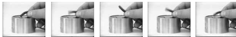
FIGURE 1. Snapshots of shape change of a magnetite load PDMS elastomer due to modulated magnetic field. The frequency of the field is 40Hz.
