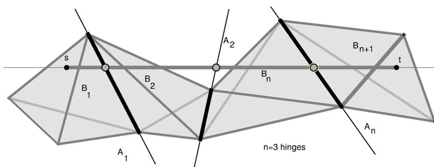
FIGURE 1. A body-and-hinge chain in  $R^3$  with  $n = 3$  hinges, four bodies (visualized as tetrahedra) and two marked points  $s$  and  $t$  on the end-bodies. In a maximum reach position, the axes meet the *oriented segment*  $st$  in the natural order.
