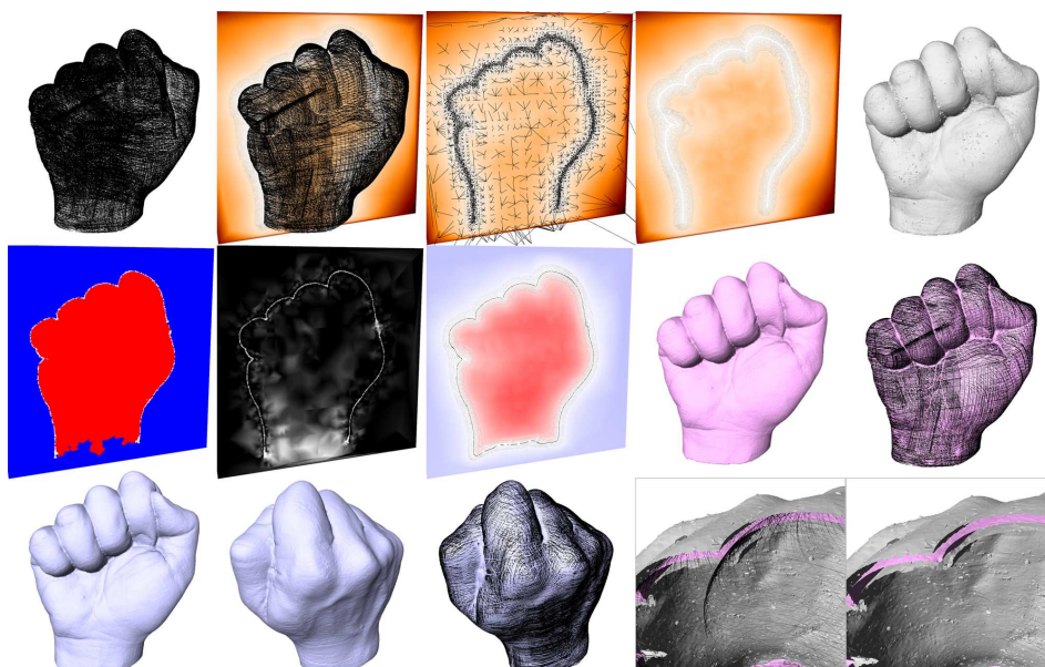
FIGURE 2. Plaster Hand. Data scanned with a Kreon laser scanner mounted on an articulated arm; the 18M point sampling is very anisotropic as it was obtained by manual sweeping of a 1D contact sensor. Top: input point set (with a big hole at the bottom and others due to occlusions between the fingers), point set and 2D cut of unsigned function, same 2D cut with nearby edges of the coarse mesh, same 2D cut alone, and full \epsilon -band. Middle: 2D cuts of sign guess (red for inside, blue for outside and white uncertain), confidence (which decreases in the holes), signed function after smoothing, isosurface of the robust unsigned function obtained by marching tetrahedra in the lattice mesh, and same isosurface superimposed with input points. Bottom: views of the reconstructed surface obtained by Delaunay refinement without and with points added, and cut view of the \epsilon -band with the reconstructed isosurface of the signed function inside, with and without the input points.
