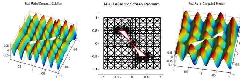
FIGURE 1. Real part of the computed IPDG solution for  $k = 15$  (left); refined mesh for  $\theta = 0.1$  in Dörfler marking for  $k = 15$  (center); Real part of the computed IPDG solution for  $k = 20$  (right) .
