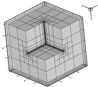
FIGURE 1. Geometric mesh on Fichera domain with  $\sigma = 0.5$ .
