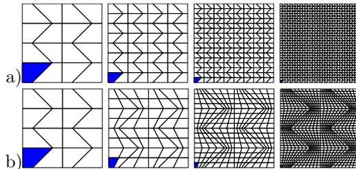
FIGURE 1. Sequence of meshes used to test convergence rates of standard DG and LSC-DG. Top: meshes obtained through self-similar refinement. Bottom: meshes obtained through bisection.
