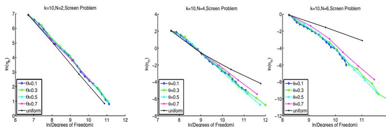
FIGURE 2. Convergence history of the adaptive IPDG method. Error estimator as a function of the DOF (degrees of freedom) on a logarithmic scale:  $k = 10, N = 2$  (left),  $k = 10, N = 4$  (center), and  $k = 10, N = 6$  (left).
