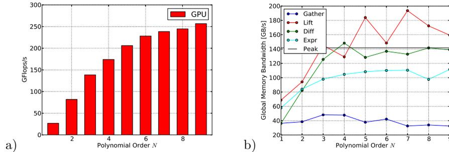
FIGURE 1. Performance of GPU-DG on Nvidia GTX295 as shown in [1]. a) Aggregate, wall-clock performance measured timestep-to-timestep. b) Achieved memory bandwidth, broken down by computational component. (Above-peak values due to texture cache effects.)
