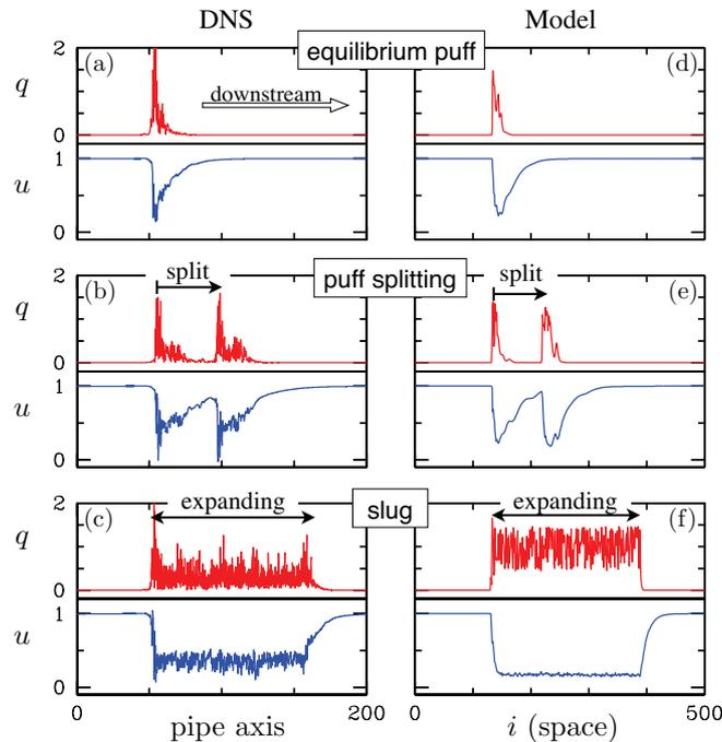
FIGURE 2. Regimes of transitional pipe flow. Left column is from full DNS. (a) Puff at  $Re = 2000$  that will decay at a later time. (b) Puff splitting at  $Re = 2275$ . The downstream (right) puff split from the upstream one at an earlier time. (c) Expanding slug flow at  $Re = 3200$ . Right column shows corresponding states from the simple one-dimensional discrete model.
