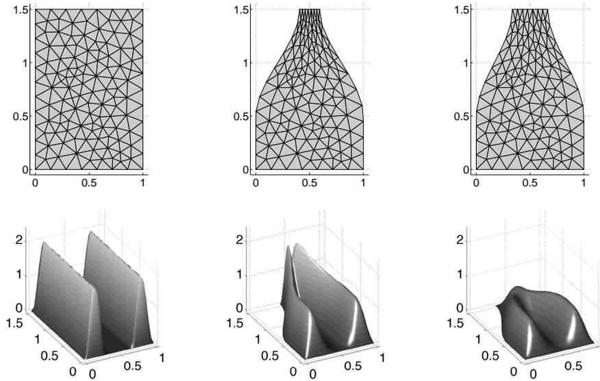
FIGURE 1. Above: the domain  $\Omega_t$  for  $t = 0$ ,  $t = 0.37$ , and  $t = 0.74$  on a coarse mesh with 131 nodes; below: the solution for  $t = 0$ ,  $t = 0.37$ , and  $t = 0.74$  on a refined mesh with 1,871 nodes.
