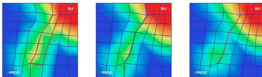
FIGURE 1. Understanding modeling choices: averaged (left), meshed-in (middle) and interface (right) approaches
