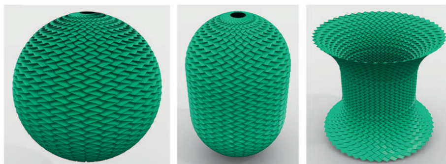
FIGURE 2. Some example generalized Miura patterns, generated using numerical optimization, approximating curved surfaces.
