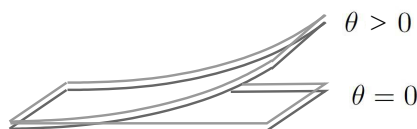
FIGURE 1. Bending of a bilayer sheet due to a mismatch of material responses to, e.g., temperature.
