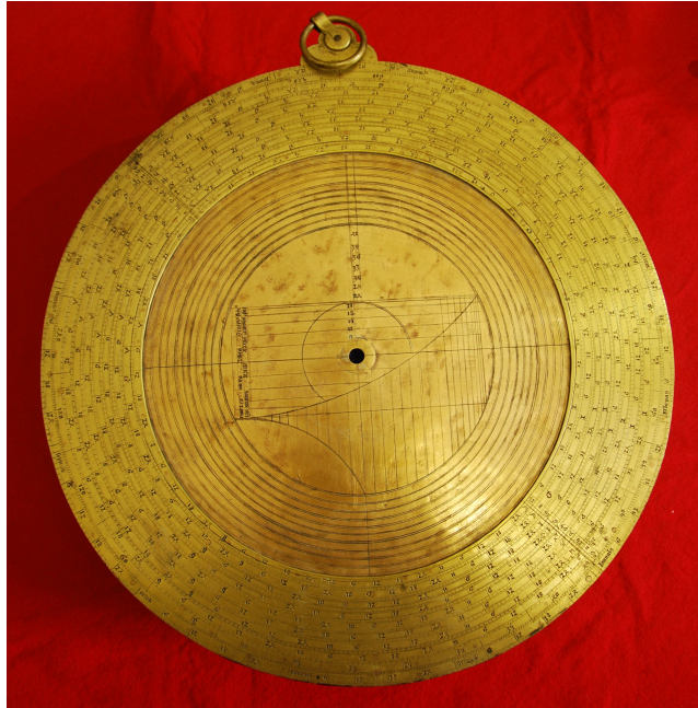
FIGURE 1. Albion ( \varnothing = 325 mm), made in central Europe in the 15th century, following the instructions in Richard of Wallingford, Tractatus Albionis (1326). Rome, Museo Astronomico e Copernicano
