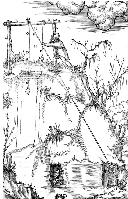
FIGURE 1. General principle of the geometria subterranea according to G. Agricola [1, p. 90]
