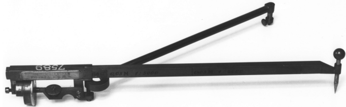
FIGURE 2. Amsler's polar planimeter
