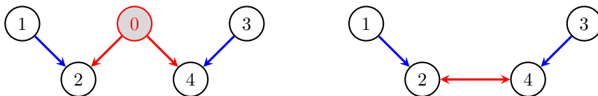
FIGURE 1. Left: a DAG with five vertices, where 0 represents a latent variable. Right: the MAG that corresponds to this DAG with 0 removed.
