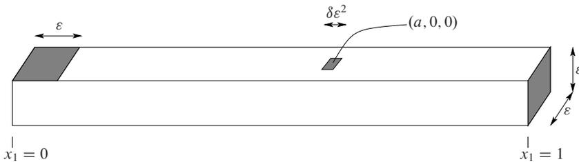
Figure 1. The domain  $\Omega_\varepsilon$ . The grey parts correspond to Dirichlet boundary conditions, the other ones to Neumann boundary conditions.
