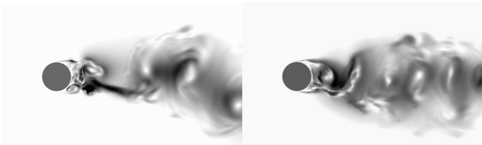
FIGURE 1. Two snapshots of the turbulence strength in the Kármán vortex street: from Large eddy simulation [15] (left), and generated by DCGAN [5] (right).
