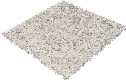
FIGURE 1. Fiber network model of paper at the millimeter scale.
