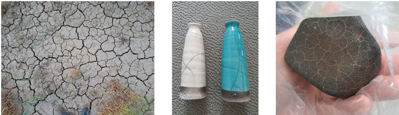
Figure 2. Network of cracks in drying mud (left), cracks in the glaze of ceramics as a decorative element (center) and cracks in the fusion crust of a meteorite (right).
