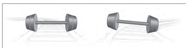
Railway wheel sets (properties of a cone).
