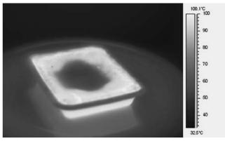
Thermal camera image of food in a domestic turntable oven, showing a distinct 'cold spot' in the centre caused by a local minimum in the radiant electro-magnetic field.
