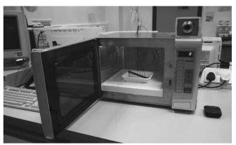
A domestic mode-stirred microwave oven with four temperature probes used to test the predictions of the model.
