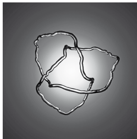
Figure 2. A knotted vortex tube of water obtained in the Irvine Lab at the University of Chicago (Figure courtesy of William Irvine)
