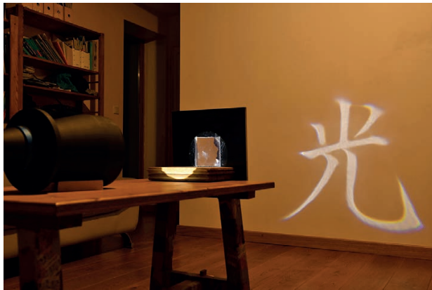
Figure 2. Lens transforming a parallel light source into a hikari
