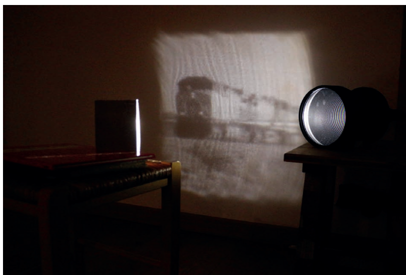
Figure 1. Mirror transforming a parallel, uniform light source into the shape of a train
