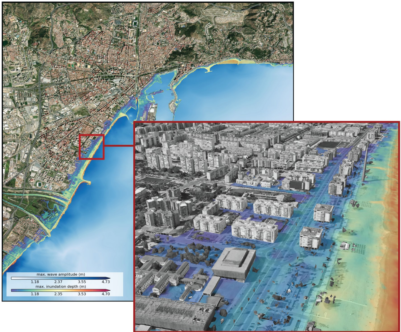
Figure 13. High-resolution inundation simulation in Málaga. (Base imagery © Google Earth, Landsat/Copernicus)
